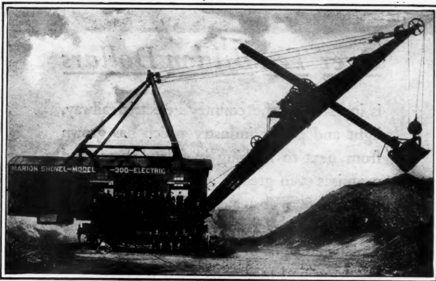
The largest one-man shovels in the world, equipped with General Electric motors, take eight dump cartloads at a bite, and can take a bite a minute.
